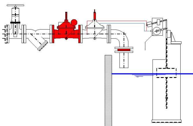
If the pressure is between 9 to 16 bar, a Hawido pressure reducing valve is required before the floating valve.
