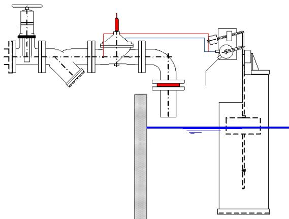
If the inlet pressure is between 4 to 9 bar, an orifice is required after the Hawido valve. The pressure will be reduced in two steps.
