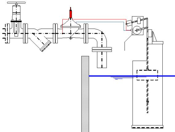
Inlet pressures from 1.5 to 4 bar the Hawido floating valve type 1600 can be used together with an opening limiter.
