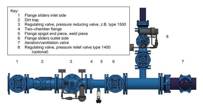
The HAWIDO must be installed horizontally with the valve cover upwards (other models available on request). We recommend that a gate valve and a dirt trap be fitted in front of the valve, as well as the mounting of an gate valve at the outlet.
