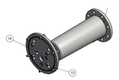
The pressure screw, pressure nut and the fibre washers are lubricated for a long duration and must not be dismantled. Dismantling the coupling and the pressure screw could possibly result in a new adjustment of the end stops.
