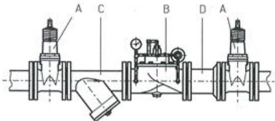
Regulating valves are normally fitted with the valve cover upwards and it is recommended that shut-off valves be fitted on both sides plus a dirt trap on the inlet side. Depending on the installation situation, a mounting adapter may also be required. Before commissioning, a check should be made that no coarse foreign bodies can penetrate into the HAWIDO.
