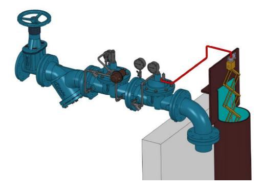
The HAWIDO must be installed horizontally (other installation models on request) with the valve cover upwards. We recommend that a shut-off valve and a dirt trap be fitted in front of the valve. Depending on the pipework construction (e.g. the piping runs upwards) a shut-off valve after the valve should also be planned. Before the installation, check that no coarse foreign objects can penetrate into the HAWIDO.
