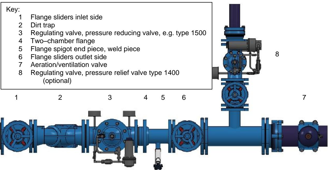
The HAWIDO must be installed horizontally with the valve cover upwards (other models available on request). We recommend that a gate valve and a dirt trap be fitted in front of the valve, as well as the mounting of an gate valve at the outlet.
